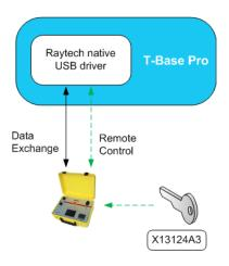
The T-Base Pro remote option of Raytech devices can be unlocked by entering a license key.
