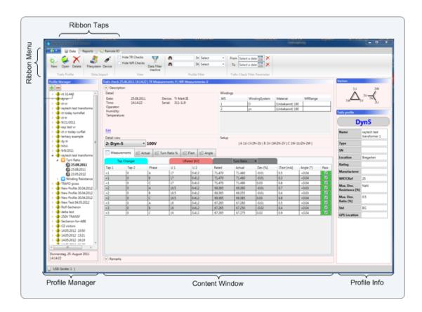
Raytech T-Base Pro is a **full multi tasking system**. For instance a measurement with long duration can be started. While it is running, the user can create new profiles, exchange data with other devices, start another measurement and so on.
