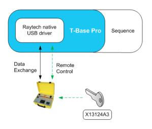
Sequence is an existing Add-On to control Raytech devices and doing complete transformer measurements in a free programmable measuring process, including winding resistance and turns ratio measurements.
