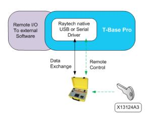
This is a basic Add-On provided by Raytech. It calls any program with a parameter on a PC. An XML file as return value is accepted.
