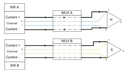
As the system cabling is different for one and two winding resistance meters, nothing changes in the control scheme of Multiplexers.
