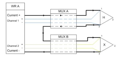
The current flow in the winding systems is exactly the same.
