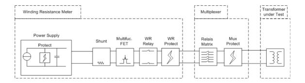
The crowbar circuit called 'Mux Protect' avoids flashover in the relay contacts of a Multiplexer. This circuit shortens the input when voltage rises above 600V.
