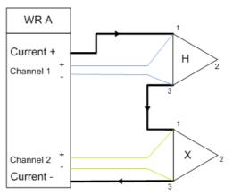
The table sais to put Current + to H1, a jumper from H3 to X1 and put Current – to X3. Channel 1 is putted from H1 to H3 Cahnnel 2 is putted from X1 to X3
