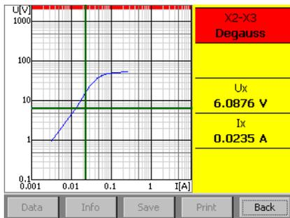
8. The *Excitation curve* for the second winding is drawn on the same diagram.
