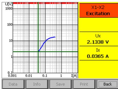
6. The *Turns ratio* is measured at different voltages below the detected *Knee point*. Please keep holding down the *Surveillance Switch* during this phase as the voltage might be increased above 50 V depending on the detected *Knee point*.
