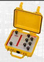
Battery and mains operated. Heavy duty protection circuitry. Color touch screen. 2 independent measuring and temperature channels. Internal printer. Fast discharge unit. Internal «Heat run test» software available. USB interfaces. Mounted in a rugged case. Fully automatic demagnetizing circuit.
