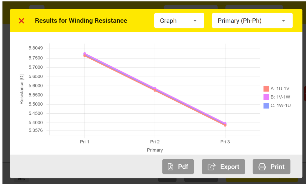
Figure 59: Winding resistance graph results view
